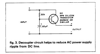
regulation will cause erratic characters. Long-term changes in supply voltage from, for example, 12 volts to 10 volts, will drastically affect the weight of the characters, and to a lesser extent, the speed. The keyer will work well with supply voltages of 9 to 15 volts. Once the operating voltage is selected it must remain at that value; if it does not, all controls will require re-adjustment.
